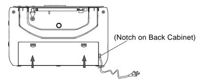
Slide the battery cover upward until it snaps back into place. Connect the AC cord to your 120V 60Hz AC outlet.
